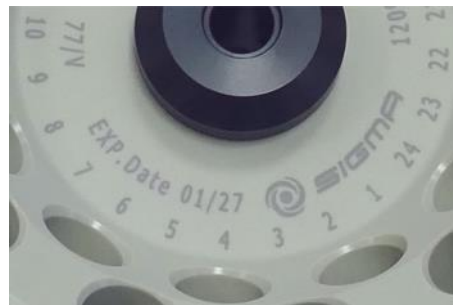
Fig. 4: Different service life – engraving on the bucket/rotor
