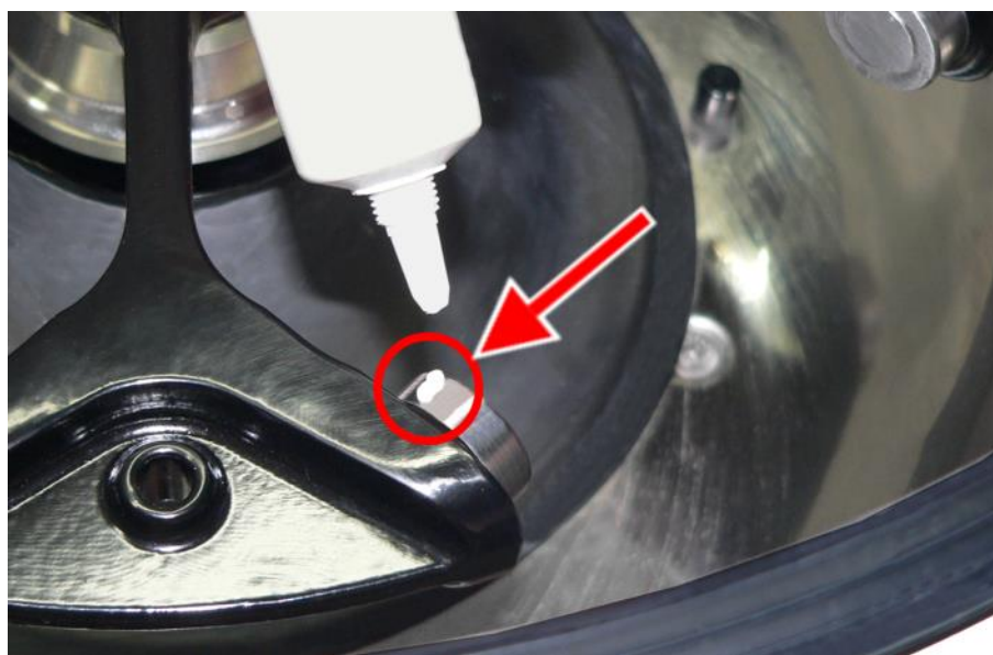
Fig. 22: Sufficient quantity of grease for one bolt
