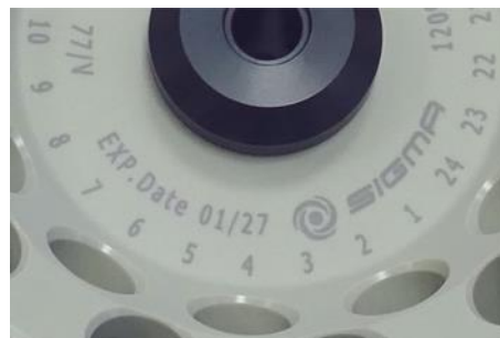
Fig. 4: Different service life – engraving on the bucket/rotor
